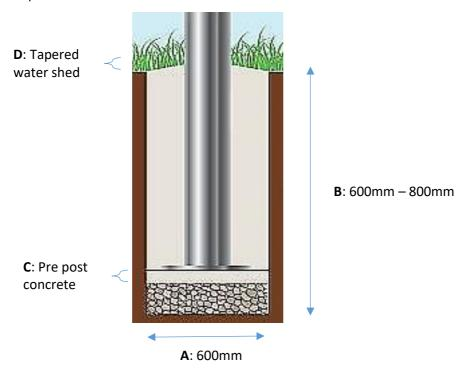
Ensure post is straight and level before continuing the concrete. To avoid water sitting around the post base, finish with a tapered water shed (D). Allow concrete to set.
